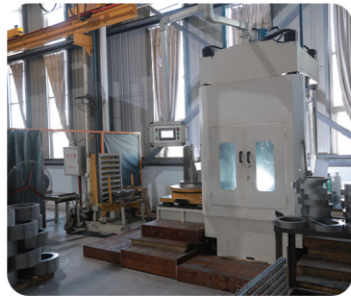
Stator core lamination and auto-welding
