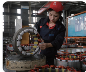
Exciter stator coil inserting
