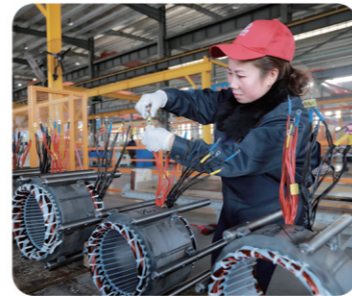
Stator coil inserting
