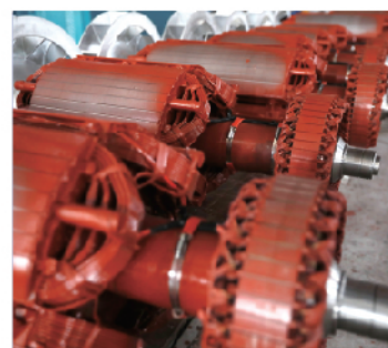
THREE-PROOF PAINT TREATMENT
