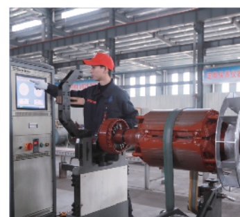
DYNAMIC BALANCE TEST
