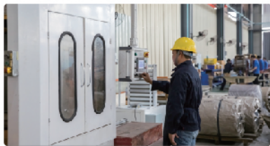
Stator core lamination and auto-welding
