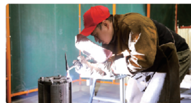
Rotor core welding
